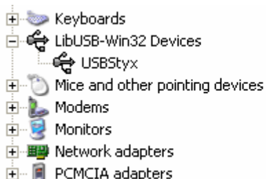
Figure 25. USBStyx Driver Verification Using Device Manager
